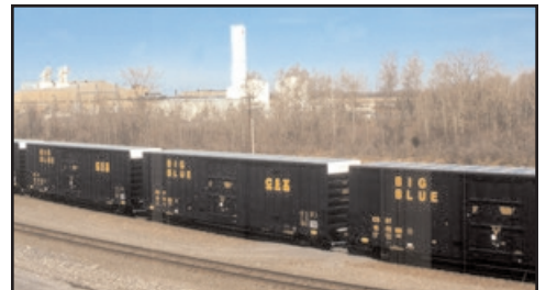
To protect paper lading during transport, CSXT recently purchased 220 60-foot, Plate F "Big Blue" boxcars from Gunderson.
